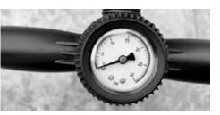
**STEP 6:** Use a pump with gauge, inflate the kite to the recommended 6 psi.
