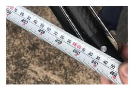
For the 8.5 rig, around 6100mm. For the 9.5 rig, around 6600mm. These are only benchmark settings, rake varies depending on the weather conditions.
