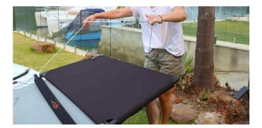
**To remove wings:** Undo the retaining fast pin, pull the rear wing bar out and away from the hull. When clear of the 2 attachment pins, lift the rear wing bar upwards. Then slide the front of the wing outwards and away from the hull – the wing should come away easily.
