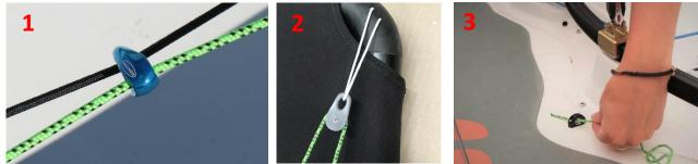
5. Return the cord to the wand tube and thread the cord up the wand as shown. When finishing the closed loop, it is best to push the wand down the tube, so the top of the wand is just below the entry and exit slot for the rope. Then insert the tail of the wand rope in and push the wand up.
