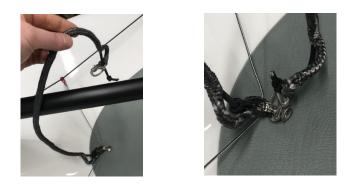
5. To adjust the shock cord tension. Loosen the knot on the shock cord, and re-tie the knot in the desired location.
