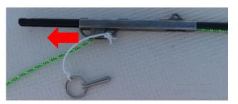
3. Push the wand tube assembly into the groove on the bow mechanism and push the fast pin into the holes to connect both components together.
