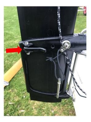
2. Attach the horizontal foil by aligning the pins, press the push button in and pushing it up into place. Make sure the push button is fully engaged before going sailing. The button will sit flush on the outside surface of the rudder.
