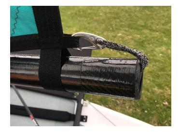
2. On the topside of the boom there is a v-cleat, the rope passes through this and can be adjusted as necessary.
