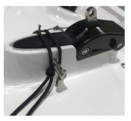
4. Once in deep water, open the clamp and push the daggerboard fully down and insert the retaining pin through the hole in the foil case and daggerboard. Pull the shock cord attached to the retaining pin over the rudder and over the other end of the retaining pin.
