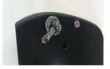
4. The excess rope can be hooked over the knob at the end of the tiller.
