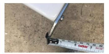
2. Walk to the head of the mast and measure the distance to the top of the carbon mast (not the plastic head fitting).
