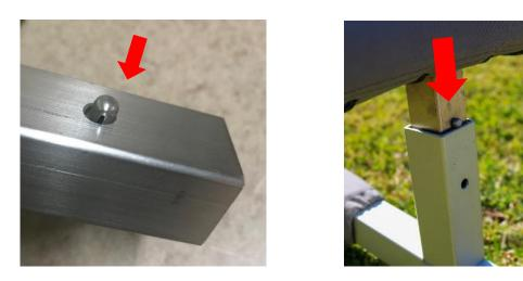
5. Attach the handle by again pushing the spring clip in and inserting it into the tube at the very front of the trolley. The spring clip will click into the hole.
