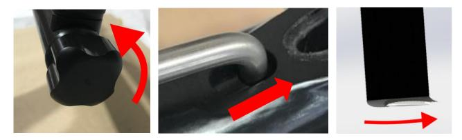
For a base foiling setting, keep the rudder pin to the front of the slot. This will give the stern of the boat maximum lift for easy foiling.
