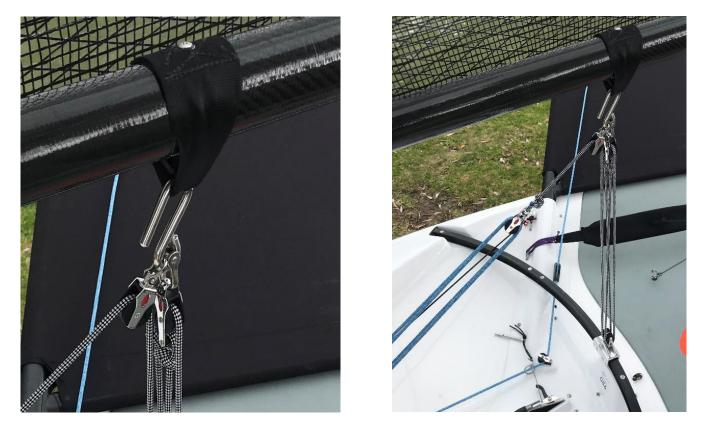
When the vang is applied, the luff is free to move down the mast, which applies both luff and leech tension at the same time. This greatly simplifies the controls and gives more time to concentrate on sailing the boat.
