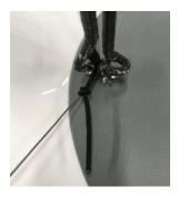
Always make sure the shock cord across the tiller is loose enough as this helps the boat to round up if you do go overboard.
