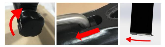
Rotate the knob anti-clockwise to reduce angle of attack on the rudder lifting foil, to sink the stern of the boat during foiling. The Rudder Pin will move towards the back of the slot.
