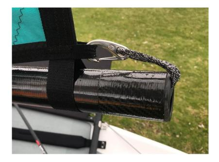
2. Insert the yoke end into the webbing loop on the tack of the sail and clip the yoke onto the mast. Ensure the webbing is positioned in front of the boom hook.
