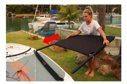
2. Lower the rear bar into position and push the bar over the inner pin.
