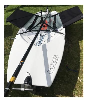
4. Raise the mast and position the mast base onto the mast step pin attached to the boat.
