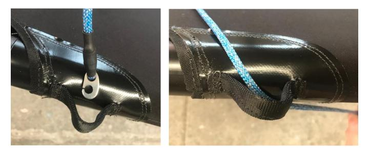
2. On the underneath side of the wing (where the orange stripes are) near the aft and inner wing bar, there is a sister clip. Pull both sister clips together and connect them.
