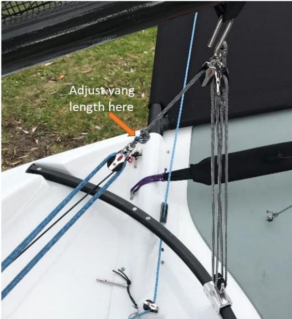
The vang is the most important rig power control. It should be set so that it can be pulled on very hard if required, completely flattening the sail for strong winds.
