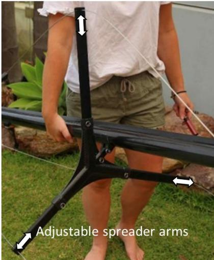
There are three adjustable spreader arms fitted to the spreader system on the mast. Without these, the mast bends a lot in the middle which causes the sail to become very flat, the leach lays off and the sail lacks power. None of which is good for foiling.
